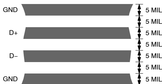
Figure 21. Typical Arrangement of Signal Tracks
