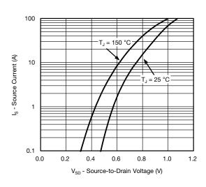
Soure-Drain Diode Forward Voltage
