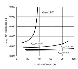
On-Resistance vs. Drain Current and Gate Voltage
