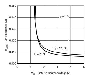
On-Resistance vs. Gate-to-Source Voltage
