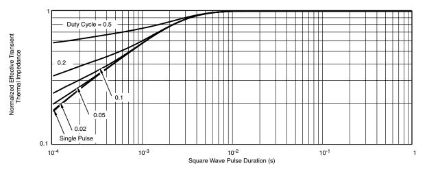
Normalized Thermal Transient Impedance, Junction-to-Case
