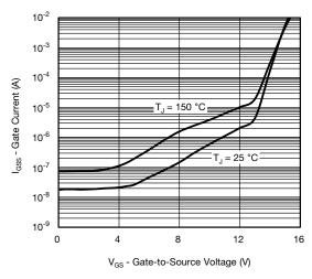
Gate Current vs. Gate-Source Voltage
