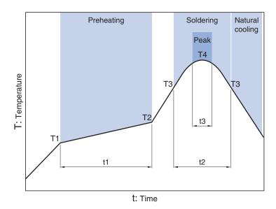
Soldering Peak Temp. Time Time Temp. Time T2 T4 Т3 180°C 90 to 120s 230°C 255°C 10s max. 40s
