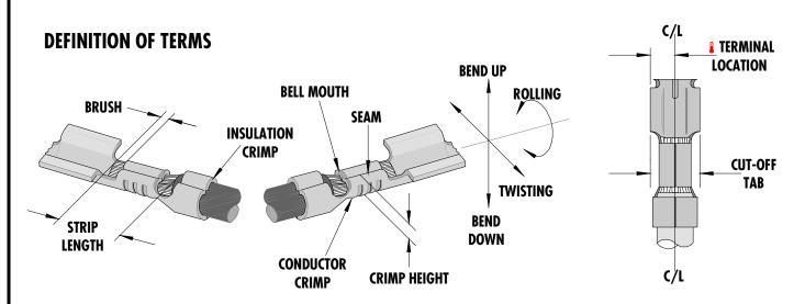
Iterminal is to be centrally located between the two (2) cut-off tab edges by one half of the total cut-off tab tolerance. This illustration is a generic terminal representation and not an exact image of any terminal listed in the scope.
