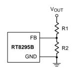
Figure 1. Output Voltage Setting
