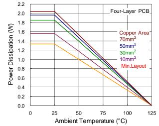
Figure 7. Derating Curves for RT8295B Package
