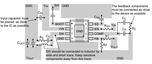
Figure 8. PCB Layout Guide
