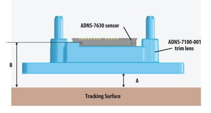
Figure 2. Optical system assembly cross-section diagram
